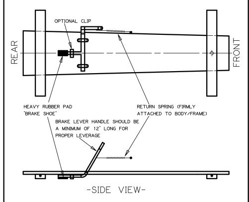
"BRAKE SHOE" TO BE LOCATED IN CAR'S CENTERLINE TO PREVENT CAR VEERING TO SIDE WHEN BRAKE IS APPLIED.
